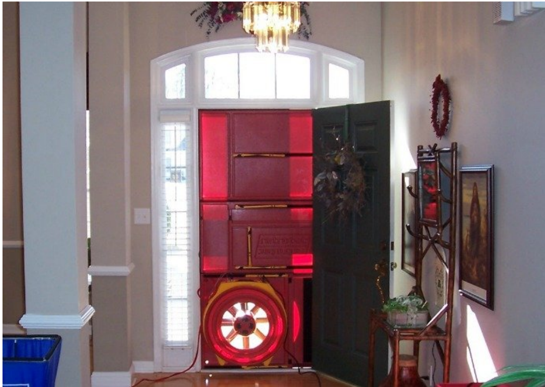
Figure IA.3. Examples of Green Certification Technical Standards. This figure shows two examples of green certification technical standards. Panel A illustrates the specifications in inspecting the roof deck above the attic as part of the on-site inspection procedures for California HERS Ratings. Panel B displays an example of the blower door test inspection.
